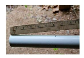
Since we wanted both cat and dog feeders, we made 6-inch and 12-inch feeders, marking with a Sharpie pen directly on the PVC where the cuts would be made, as well as where the holes would be drilled.
